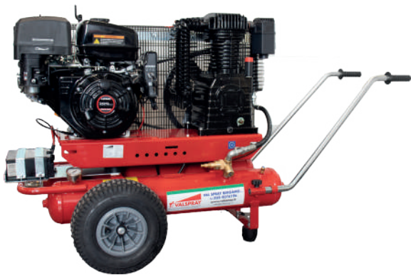
BELT DRIVEN AIR COMPRESSOR WITH 3 HEADS SUITABLE TO POWER MINI SANDBLASTERS
