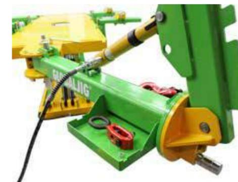
Shooting positions with double rotation, vertical and horizontal to find the right direction, and it is equipped with a practical tool drawer and a hydraulic set.
