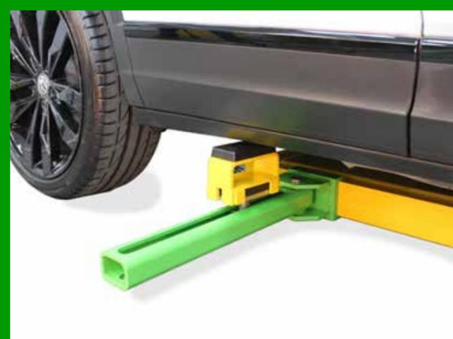
The adjustment and the choice of the height of the four sill clamps is made with the help of an air gun that speeds up the fixing operations of the car and a quick disassembly at the end of the repair operations.
