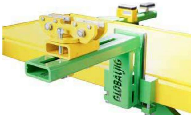
With the wide and fast height adjustment of the sill clamps it is possible to fix and lock any type of vehicle that has the edges of the crests from a minimum 89 mm to a maximum of 308 mm and it is therefore possible to apply and use on the bench any type of system computerized electronic measurement.
