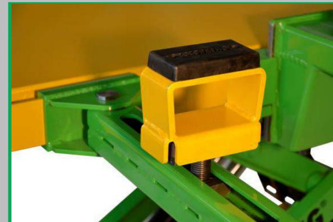
**Metal Spacers** with Rubber Pads supplement those provided on the adjustable crossbars to reach taller vehicles in order to lift the vehicle either from rocker panels, chassis frames or mechanical cross members of higher vehicles and SUVs.
