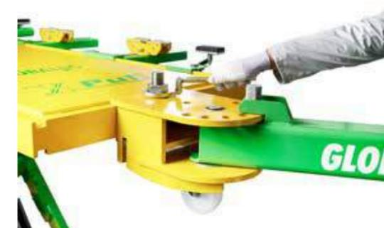
The pull arm is powerful and removable, it is applicable at any point of the frame, with the special key supplied you get a quick and secure tightening, to pull and straighten cars in any 360° direction.
