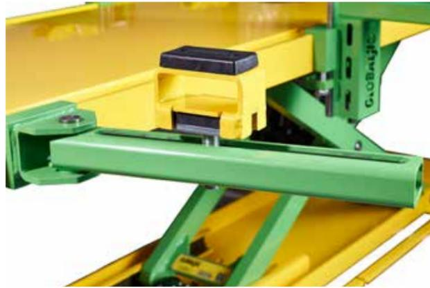
The adjustable brackets are always mounted on the frame, on which you use the sliding rubber pads adjustable in height manually, even when you are positioning the car, and those stackable are used to lift vehicles with higher bodies.
